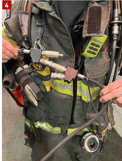
4. EBSS allows for buddy breathing. (Photo courtesy of Firefighter Air Coalition/Shur-Sales & Marketing-Fire Division.) 5. Heads-up display lights (the second red light is a battery indicator). (Photo courtesy of Firefighter Air Coalition/Shur-Sales & Marketing-Fire Division.)
