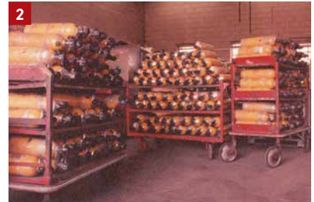
2. Refilling SCBA bottles at a remote facility and transporting them to a high-rise building fire is both labor intensive and time consuming and not a sufficient on-scene air supply system. When elevators are rendered inoperable, a stairwell bottle brigade will have to carry the supplemental cylinders up to FwS. (Photo by James Murtagh.)
