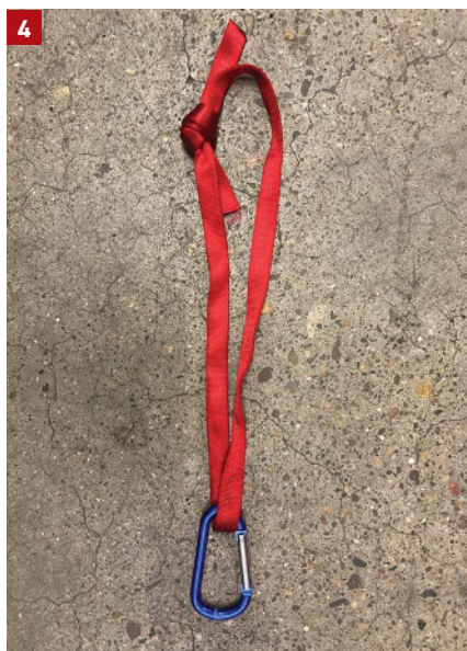
4. & 5. Critical improvements don't need to be expensive or complicated. AFR's SCBA bottle carrying strap is simple; just girth hitch the valve stem and clip it to the back frame carrying handle. The straps are sized so the bottle rides next to the back frame and at the firefighter's waist. Carrying equipment hands free is one of the best ways to minimize firefighter fatigue while ascending stairways.
