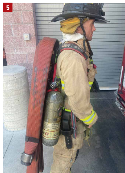
4. & 5. Critical improvements don't need to be expensive or complicated. AFR's SCBA bottle carrying strap is simple; just girth hitch the valve stem and clip it to the back frame carrying handle. The straps are sized so the bottle rides next to the back frame and at the firefighter's waist. Carrying equipment hands free is one of the best ways to minimize firefighter fatigue while ascending stairways.
